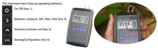
The instrument starts if you briefly depressing the key 1. After the turn on the display show for a short moment the measuring range in hPa. The instrument can use directly after turn on: The lower display show the same flow velocity as the LUGA instruments. No additional programming necessary.
