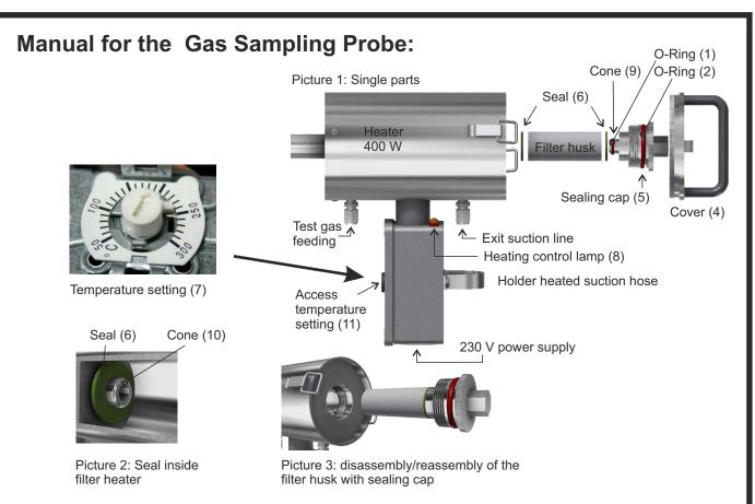
**Heater 400 W:** The probe is equipped with a high performance coil heater, which heats the exhaust pipe and the rear segment of the filter. The default value for the temperature of the filter is 200 °C. By opening the access (11) can be set a new temperature with the knob (7) (setting filter: desired temperature + 50). More than 250 °C should not be set.
