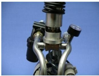
With the montage is following to heed: the two lateral screws (A) must be placed on the surfaces (F) of the square-head bolt. Use the hand wheel to place the surfaces in the corresponding position. Fix the screws (A) on the surface. Afterwards fix the engine with the socket screw (B) on the valve. The engine must now fixed solidly on the low edge of the valve.
