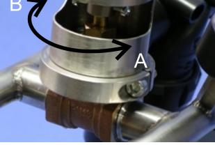
(A) more gas flow, valve turns clockwise, valve closed, green LED
