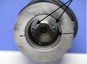
Screws (A) to fix the Ventil stem
