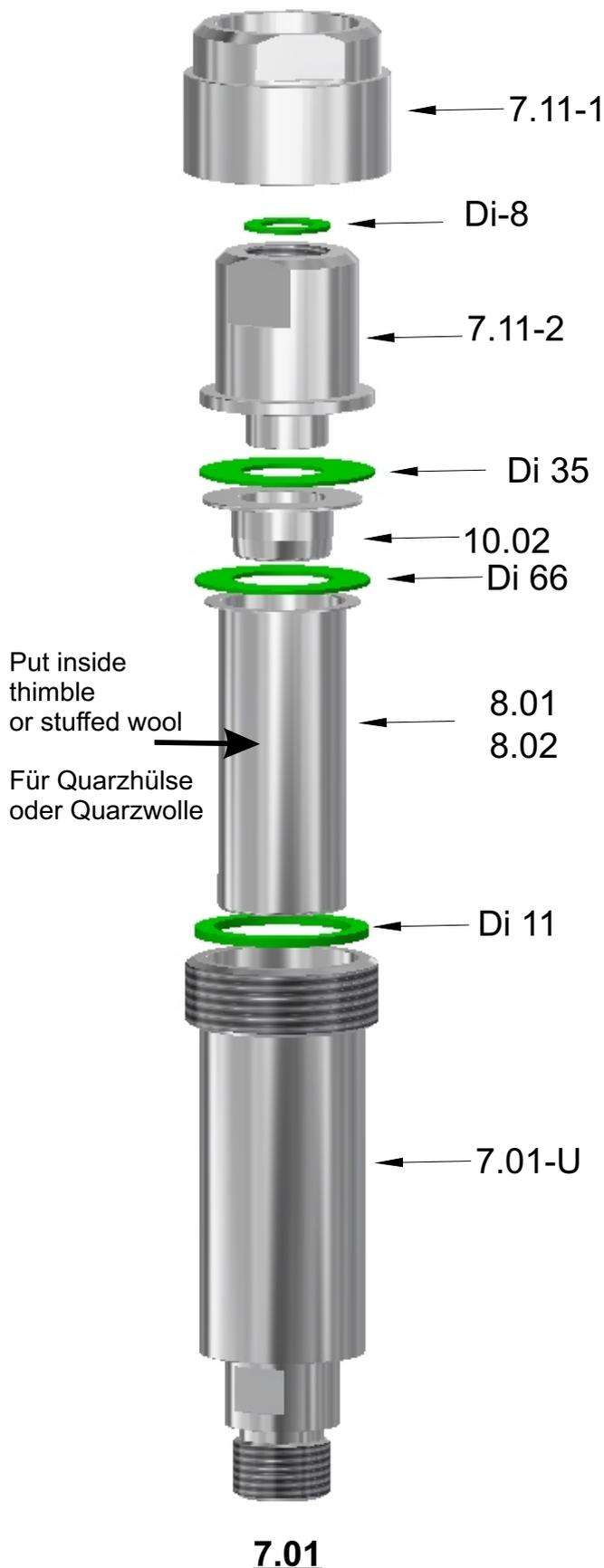
This filter device is for manual dust measurement in flowing gases and gravimetric determination of dust load if the dust content is lower than  $1000 \text{ mg/m}^3$ : The separator consist of the filter housing for stuffing with quartz wool or thimbles
