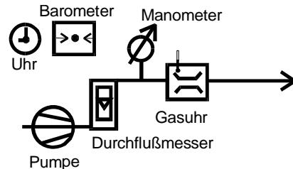
In standard situations, the flowmeter is in front of the gas meter and behind the gas tight pump. What must indicate the flowmeter if 5 m<sup>3</sup>/h should flow through the gas meter for isokinetic sampling:
