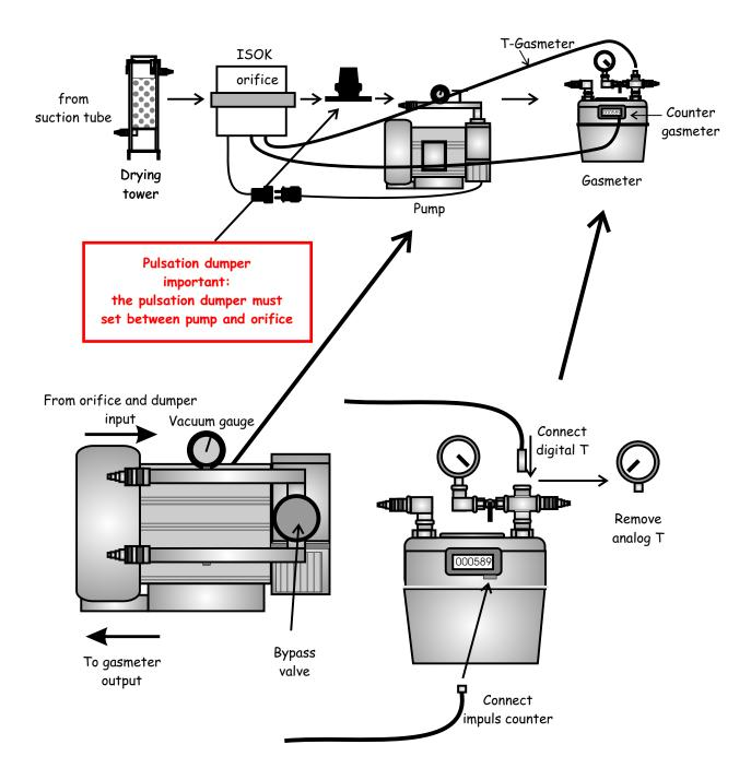
An optimal regulation is reached, if the pump is driven in the middle speed-range. The so-called "pump-volume flow rate" should set between 1,5 - 3 m<sup>3</sup>/h. The "sample volume flow rate" (from suction-side to pressure-side) is not meant with it! In case that the sampling volume flow rate through the sampling line should less as the pump volume flow rate in the middle range, the bypass-valve must be opened.
