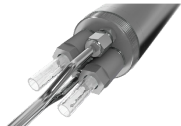
Picture 1: On the input side there is the S-pitot pitot tube for flow measurement (see instructions for S-Pitot) and a thermocouple type K (NiCr-Ni) for measuring the channel temperature. Furthermore, there are two screw connections for mounting the adsorption traps in front.
